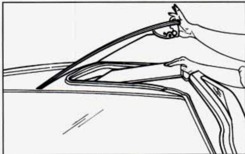
1. Start with the panel marked DRIVER FRONT. Unlatch the driver-side T-top, raise it halfway and close the latch handle.
