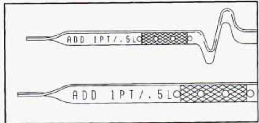
4. If the fluid level is in the acceptable range, push the dipstick back in all the way.
