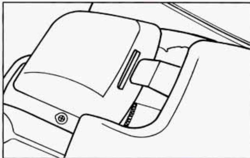
3. Remove the two side pieces of the boot cover by lifting the rear of cover and sliding them out of their slots.
