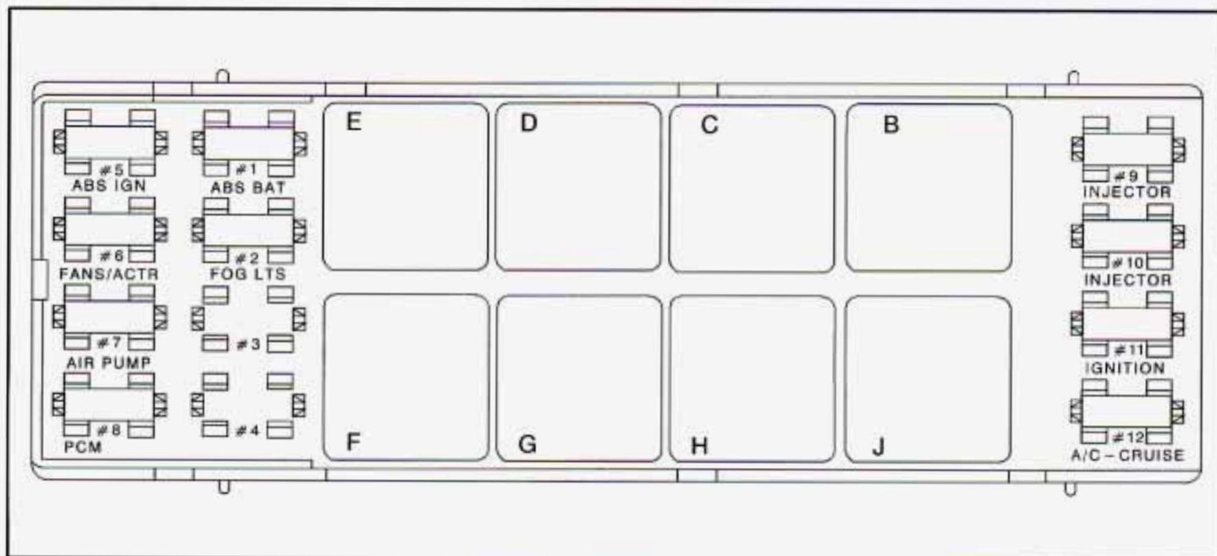
1. **ABS BAT:** Electronic Brake Control Module
