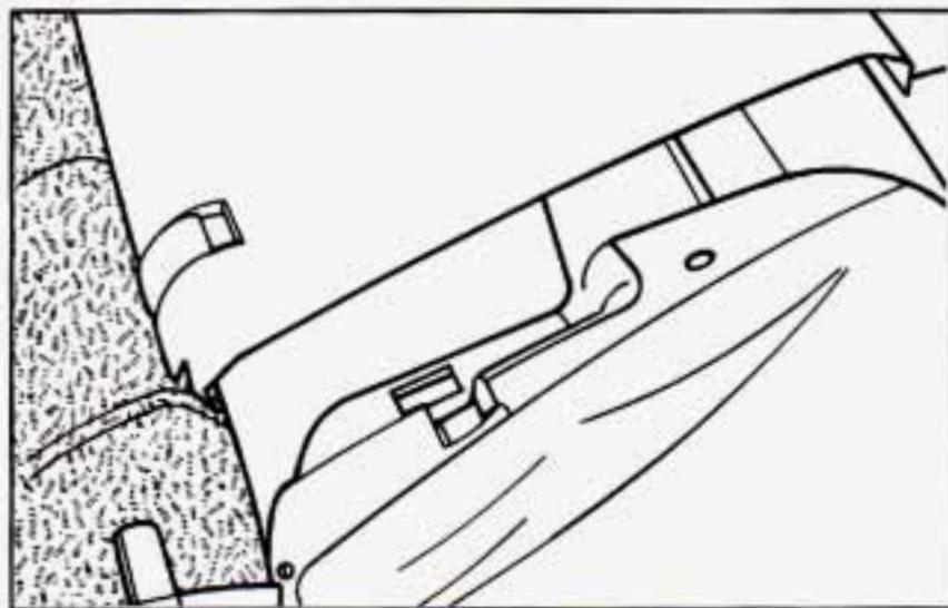
3. Install the middle section of the cover by sliding tabs into slots on right side cover. Lower the cover and engage latch.
