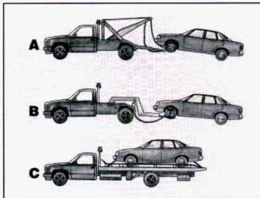
Try to have a GM dealer or a professional towing service tow your Chevrolet. The usual towing equipment is a sling-type (A) or a wheel-lift (B) or car carrier (C) tow truck.
