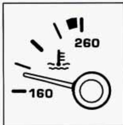
This gage shows the engine coolant temperature. If the gage pointer moves into the red area, your engine is too hot! It means that your engine coolant has overheated. If you have been operating your vehicle under normal driving conditions, you should pull off the road, stop your vehicle and turn off the engine as soon as possible.
