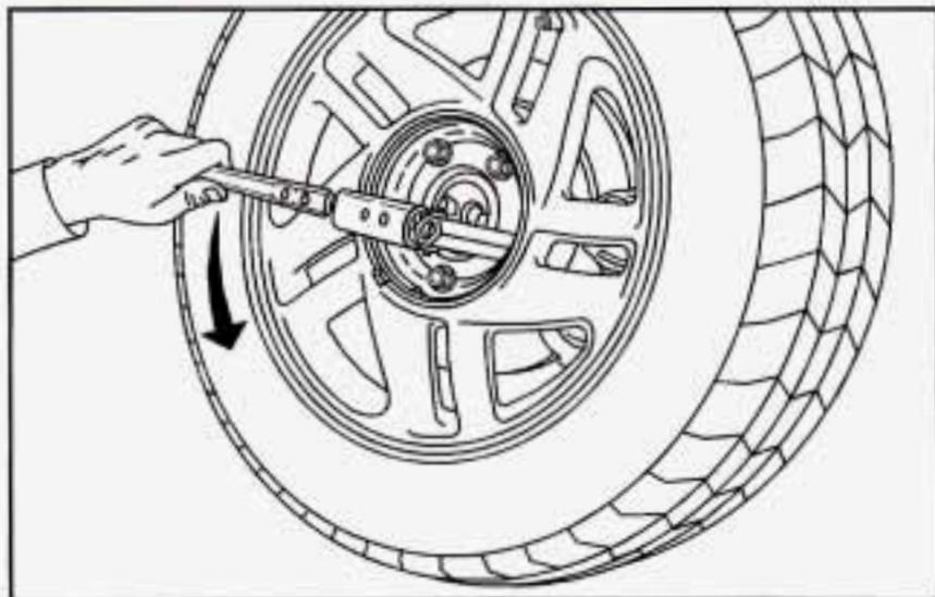
Using the wheel wrench, loosen all the wheel nuts. Don't remove them yet.
