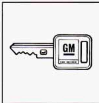
Your vehicle is equipped with the PASS-Key<sup>®</sup> II (Personalized Automotive Security System) theft-deterrent system. PASS-Key II is a passive theft-deterrent system. It works when you insert or remove the key from the ignition. PASS-Key II uses a resistor pellet in the ignition key that matches a decoder in your vehicle.
