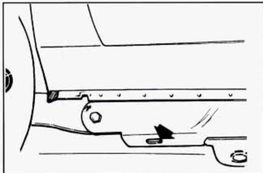
Attach T-hook chains in front of rear wheels in bottom of frame rail on both sides.
