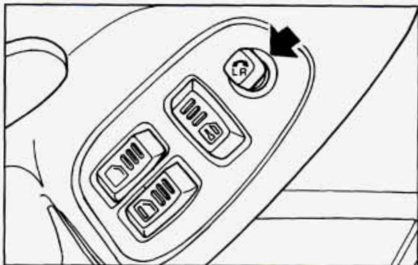
The electric mirror control is on the driver's door. To adjust either mirror, turn the switch to LEFT (L) or RIGHT (R). Then use the joystick to adjust the mirror.
