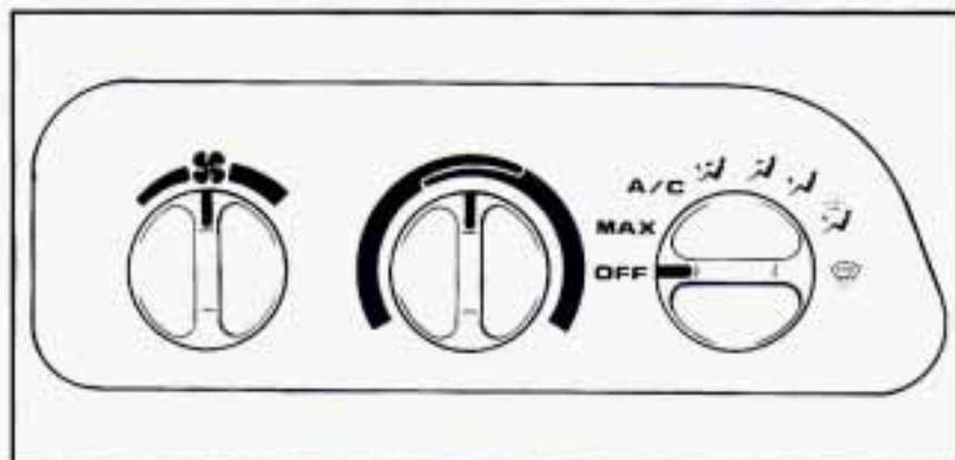
The air conditioning system uses the same controls as the heating system, except that the air control knob has two extra settings, described below. For an explanation of all the controls, see “Heater Controls” earlier in this section.
