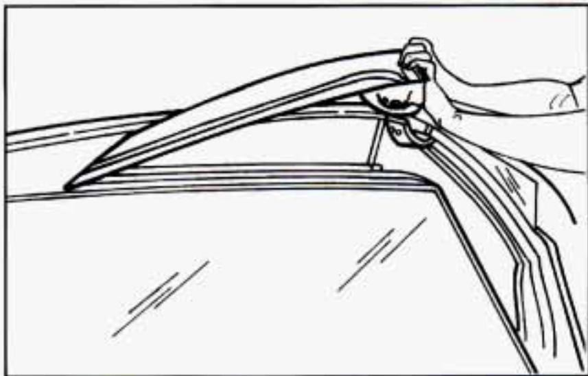
3. Open the latch and close the T-top. Check to see if there are any gaps showing. Unlatch the T-top and adjust the sunshade as required.
