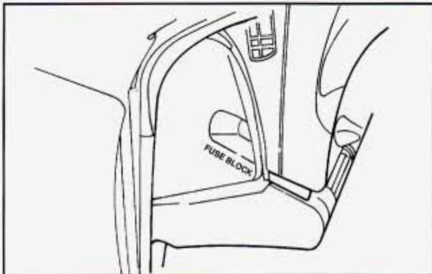
The wiring circuits in your vehicle are protected from short circuits by a combination of fuses, circuit breakers, and fusible thermal links in the wiring itself. This greatly reduces the chance of fires caused by electrical problems.
