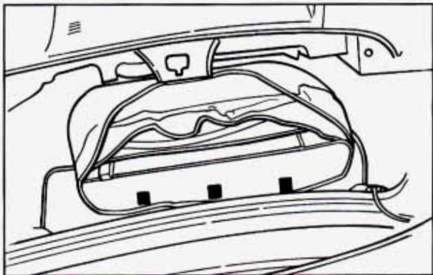
4. Store each piece of the cover in its separate compartment in the storage bag, store in the trunk and close the trunk.
