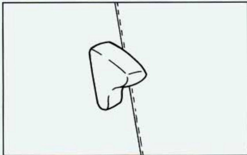
The front seatbacks fold forward to let people get into the back seat. To fold a seatback forward, push the seatback toward the rear as you lift the latch located on the lower backside of the seatback. Then the seatback will fold forward.
