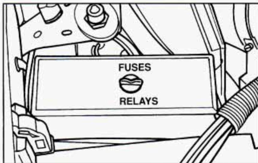
The other is in the engine compartment. Open the cover on either of the boxes to expose the fuses.
