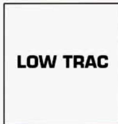
When your anti-lock system is adjusting brake pressure to help avoid a braking skid, the LOW TRAC light will appear on your instrument cluster. If you have the ASR system, this light will also come on when the system is limiting wheel spin. Slippery road conditions may exist if this light comes on, so adjust your driving accordingly. The light will stay on for a few seconds after the anti-lock system stops adjusting brake pressure or the ASR system stops limiting wheel spin.
