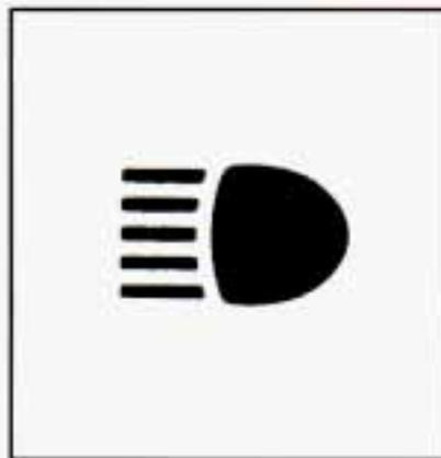
To change the headlamps from low beam to high or high to low, pull the turn signal lever all the way toward you. Then release it. When the high beams are on, this blue light on the instrument panel also will be on.
