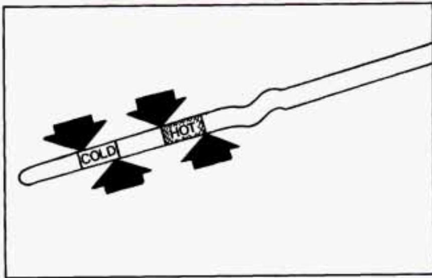
The fluid level must be in the COLD area for a cold check or in the HOT area or cross-hatched area for a hot check
