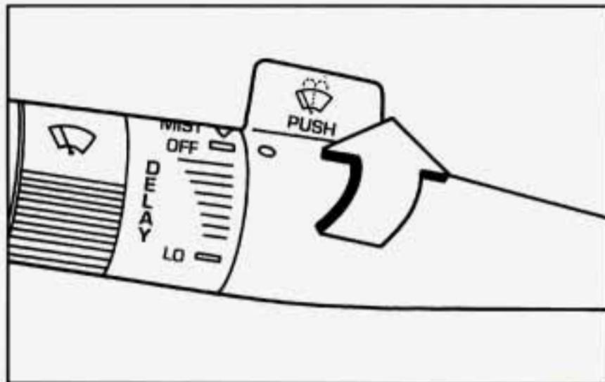
At the top of the turn signal/headlamp beam lever there's a paddle with the word **PUSH** on it. To spray washer fluid on the windshield, just push the paddle. The washer will continue to spray until you release the paddle for less than a second. The wipers will clear the window and wipe a few more times before stopping or returning to the previous setting.
