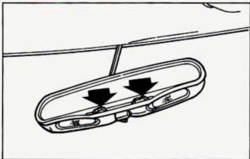
Your inside rearview mirror includes two map lamps. Each lamp has its own switch. Use the switch closest to the lamp to turn it on. The lamps will also go on when a door is opened.
