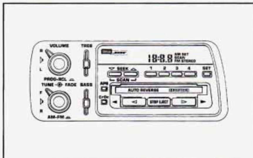
**SCAN:** The scan function uses the same two buttons as the seek function.
