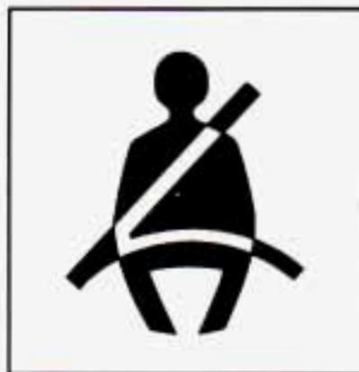
When the key is turned to RUN or START, a tone will come on for about eight seconds to remind people to fasten their safety belts, unless the driver's safety belt is already buckled. The safety belt light will also come on and stay on until the driver's belt is buckled.
