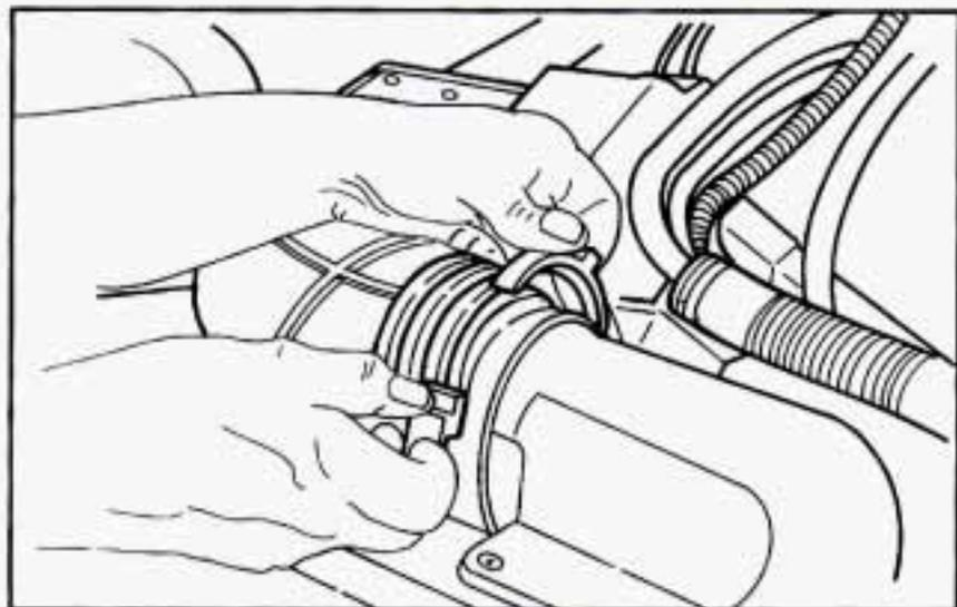
2. Disconnect the plastic clamp on the duct. Pull apart the connection.
