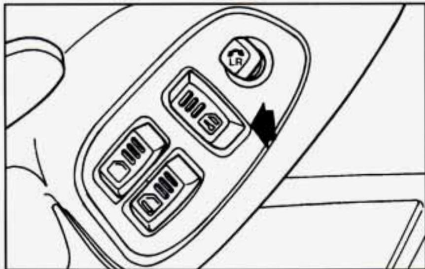
Push the power door lock switch to lock or unlock both doors at once.
