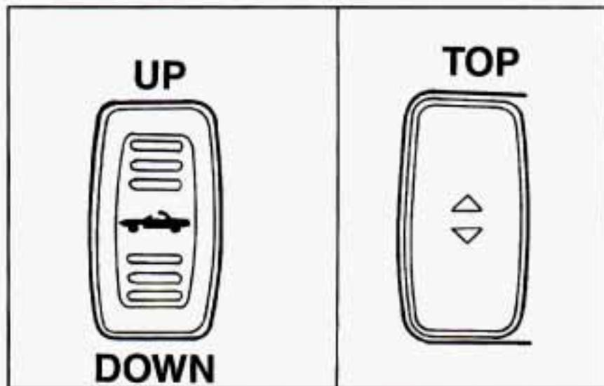
3. Be sure no one or nothing is on or around the top. Push and hold "DOWN" or ▼ on the convertible top switch. The switch is below your cigarette lighter. The top will automatically lower into the storage area.
