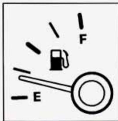
Your fuel gage shows about how much fuel is in your tank. The fuel gage works only when the ignition switch is in the RUN position. When the gage pointer first indicates EMPTY (E) you still have a little fuel left (about one to two gallons), but you need to get more right away.
