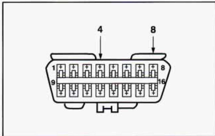
2. Insert one end of a fused jumper into terminal 8. Terminal 8 is the top terminal on the far right.
