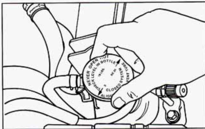
1. You can remove the radiator pressure cap when the cooling system, including the radiator pressure cap and upper radiator hose, is no longer hot. Turn the pressure cap slowly to the left until it first stops. (Don't press down while turning the pressure cap.)
