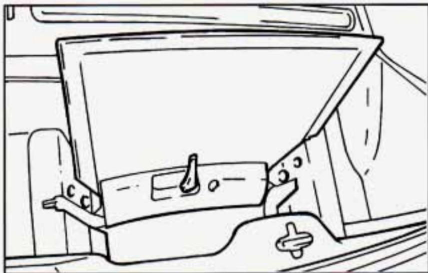
Open the close-out panel completely. Place the panel in the correct slot (driver or passenger) in the rear area of your vehicle. Make sure the handle is open and facing you when you put it in the storage slot.
