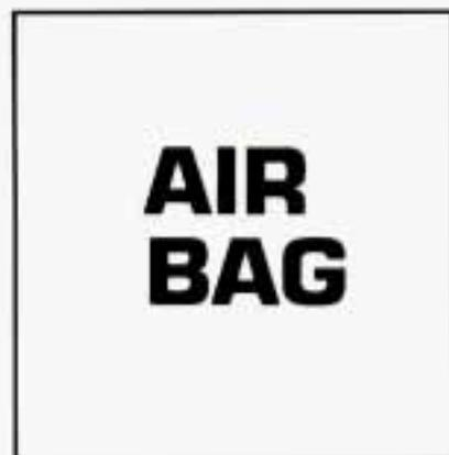
The system checks the air bag's electrical system for malfunctions. The light tells you if there is an electrical problem.
