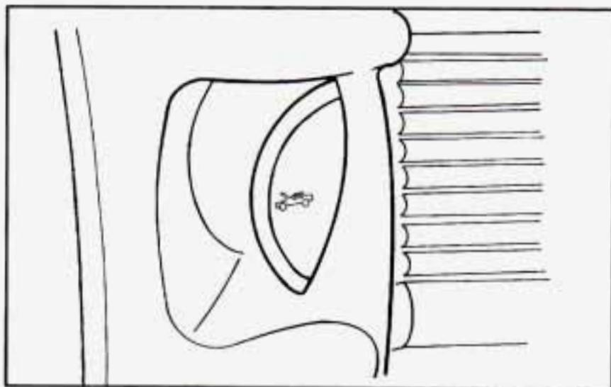
To open the hood, first pull the handle inside the lower left side of your vehicle.
