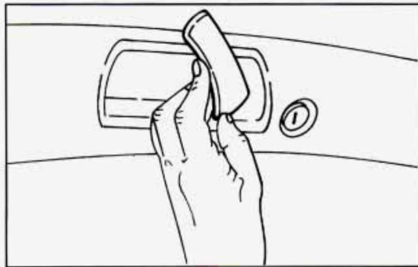
Then pull on the release handle to unlatch the panel. Lift the outer edge of the panel and pull it toward you.
