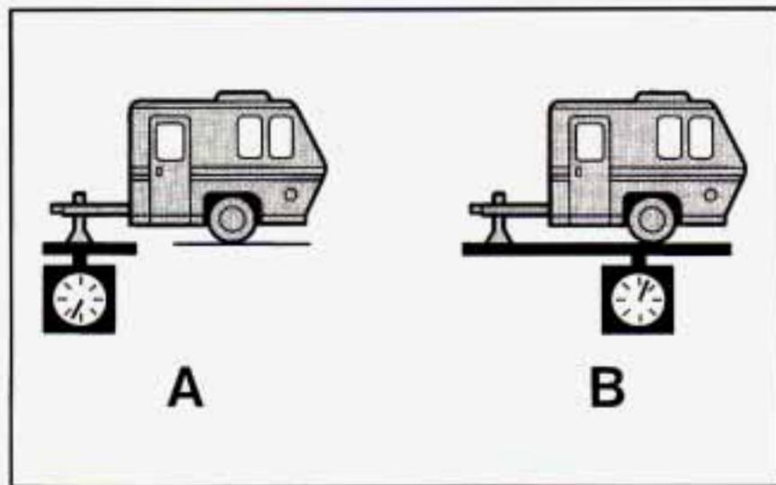
If you're using a "dead-weight" hitch, the trailer tongue (A) should weigh 10% of the total loaded trailer weight (B). If you have a "weight-distributing" hitch, the trailer tongue (A) should weigh 12% of the total loaded trailer weight (B).
