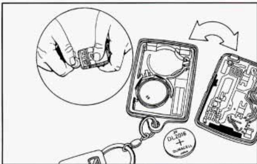
To replace batteries in the Remote Lock Control:
