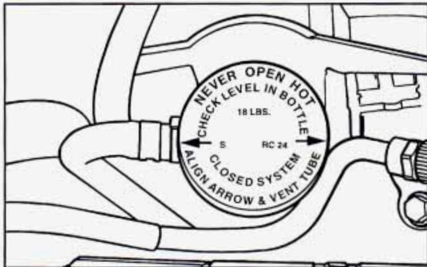
9. Shut the engine off and replace the pressure cap. Be sure the arrows on the cap line up like this.
