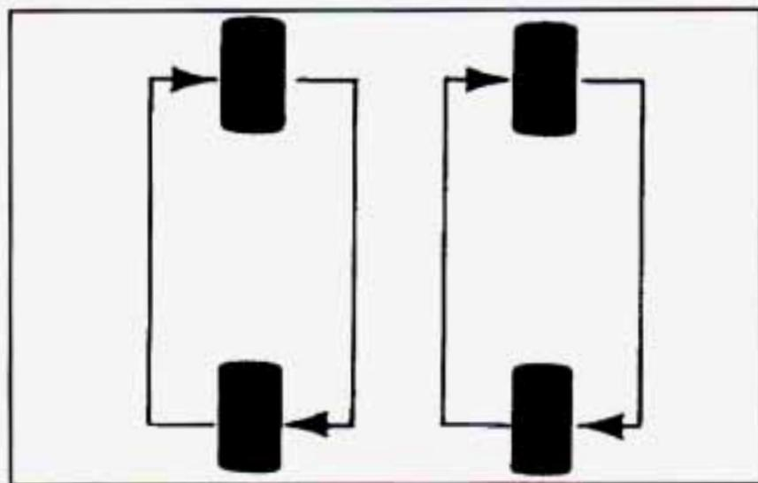
If you have P245/50ZR16 Goodyear Eagle GS-C tires, they must roll in a certain direction for the best overall performance. The direction is shown by an arrow on both sidewalls. Because these tires are directional, they should be rotated as shown here. These tires should only be moved from front to rear and rear to front on the same side of the vehicle.
