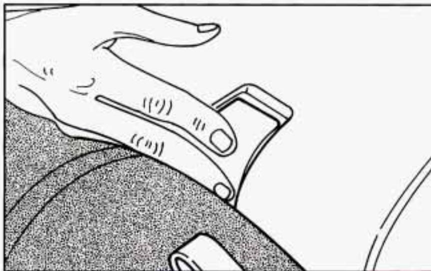
2. Open the trunk. Remove the middle piece of the cover by pushing in on the latch and lifting up on the cover.
