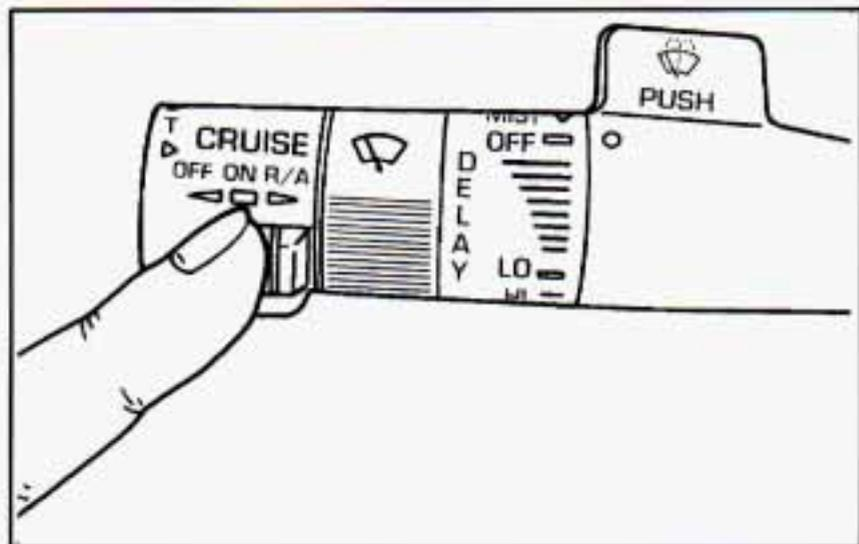
Suppose you set your cruise control at a desired speed and then you apply the brake or clutch pedal. This, of course, shuts off the cruise control. But you don't need to reset it. Once you're going about 25 mph (40 km/h) or more, you can move the cruise control switch from ON to R/A (Resume/Accelerate) for about half a second.
