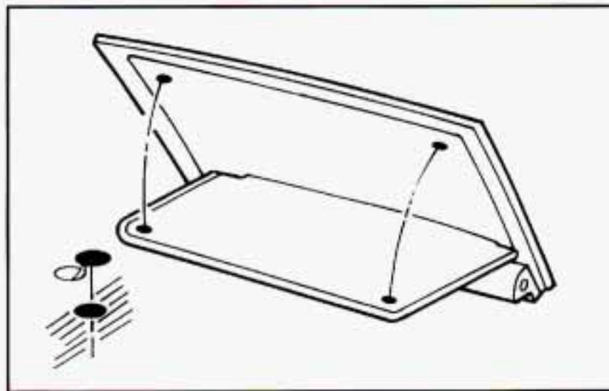
5. Pull the sunshade back a little and remove the backing paper from the velcro<sup>®</sup> buttons. Push the sunshade back into place sticking the velcro<sup>®</sup> to the glass.
