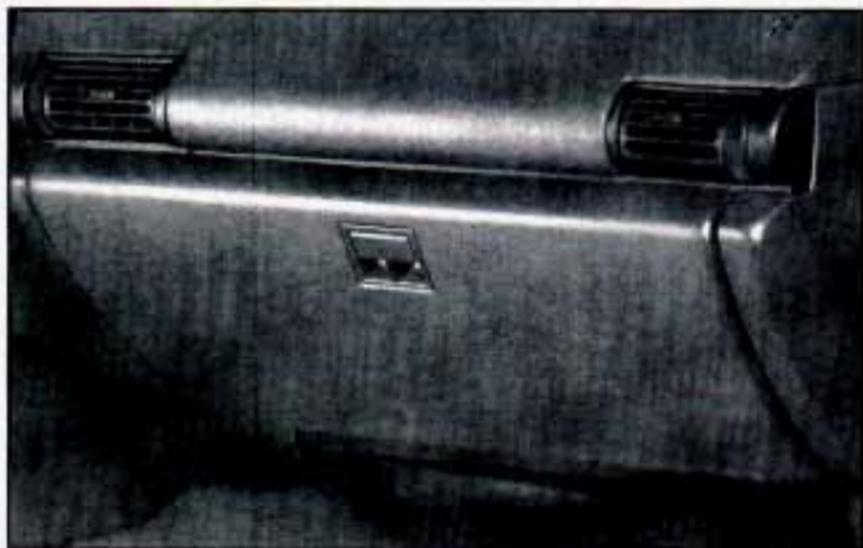
To open the glove box, lift up on the lever. Use your door key to lock and unlock it. The glove box has a light inside.
