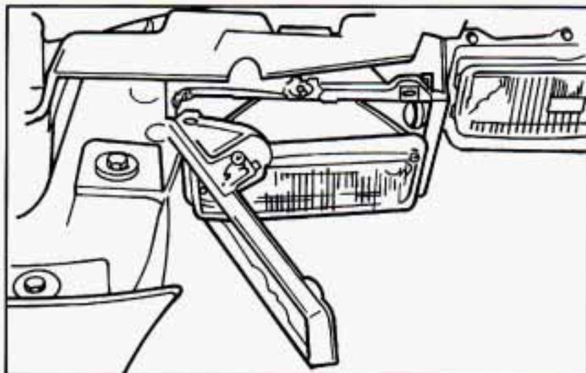
2. The aiming ring will swing open like a gate. Remove the aiming ring from the assembly. Place it face down, with the aim indicator up. Be careful not to damage the aiming bubble.
