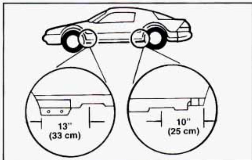
Position the jack under the vehicle. There is a notch in the vehicle's rocker flange. Raise the jack head until it fits firmly into the notch nearest the flat tire.
