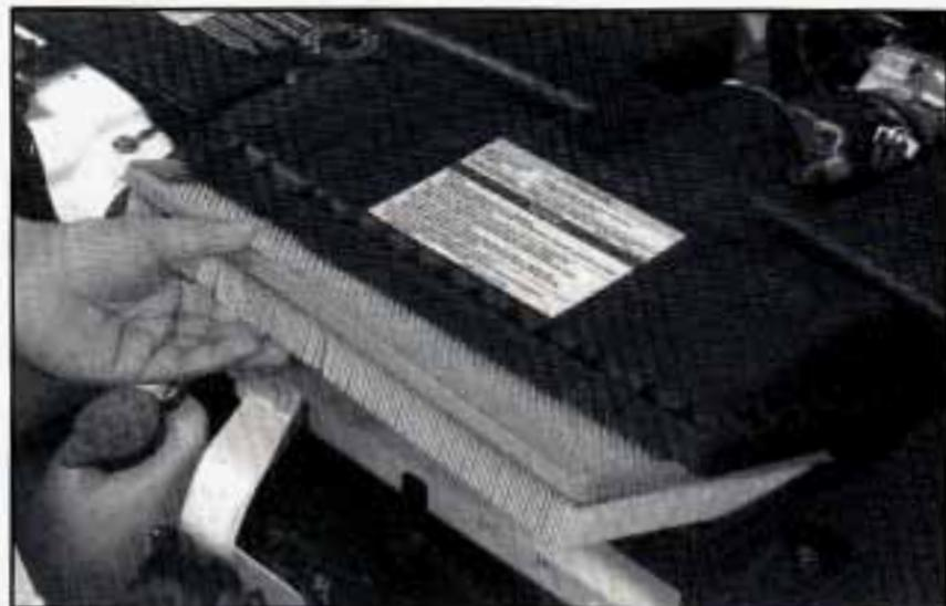
2. Lift the cover and remove the air filter.
