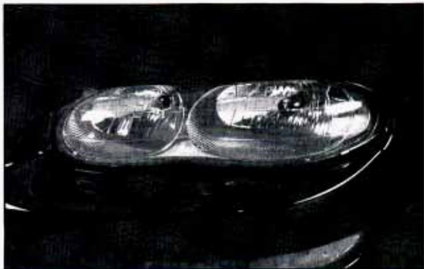
Before replacing a headlamp that does not light, check to make sure that the wiring connector is securely fastened to it.
