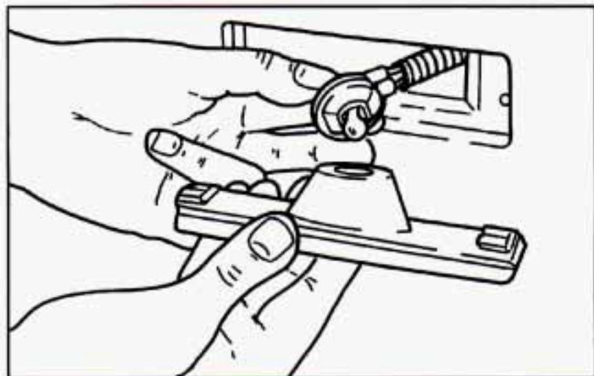
3. Turn socket to the left (counterclockwise) and pull out the socket and the bulb.
