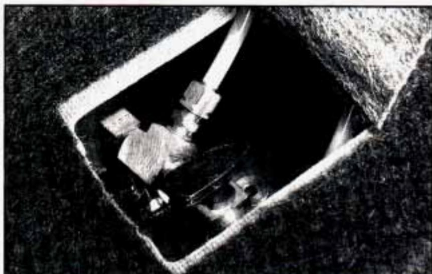
Open the hatch and find the tab along the left side trim panel. Lift up the tab and turn the valve to the left to release the hydraulic pressure. Turn the ignition key to the LOCK position. You can now raise or lower your top manually. Be sure to close the valve after installing your top so you can raise or lower it electrically later.
