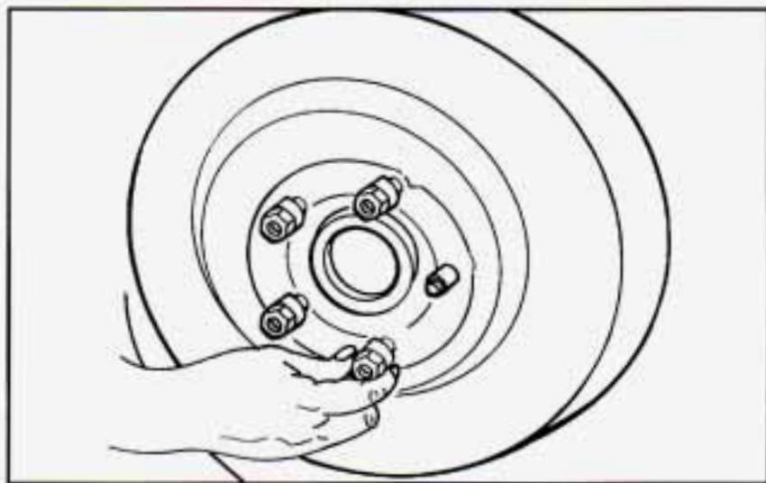
5. Replace the wheel nuts with the rounded end of the nuts toward the wheel. Tighten each nut by hand until the wheel is held against the hub.
