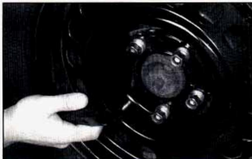
If your vehicle has optional alloy wheels, each wheel may have one locknut in place of the standard wheel nut. A special wheel lock key (removal tool) and instructions are located in the center console. Attach the wheel lock key to the socket of the wheel wrench. Remove the locking wheel nut by turning to the left.
