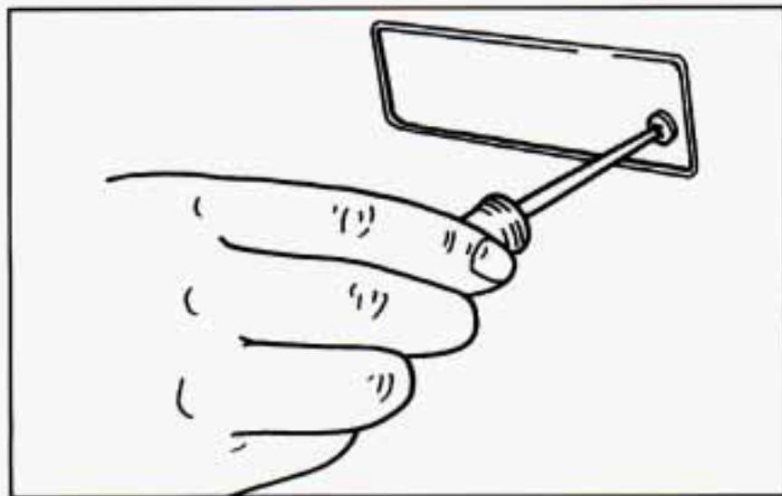
Replacing a rear sidemarker bulb:
