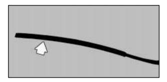
When it is cool, remove the coolant recovery tank cap and look at the dipstick. The coolant level should be at FULL COLD. If it isn't, you may have a leak in the radiator hoses, heater hoses, radiator, water pump or somewhere else in the cooling system.
