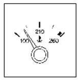
This gage shows the engine coolant temperature. If the gage pointer moves into the red area, your engine is approaching an overheating condition.
