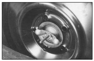
Remove the wing nut and adapter and pull out the spare.
