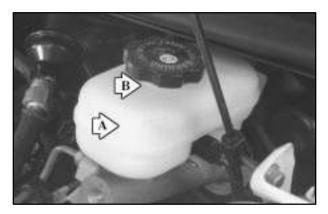
You can check the brake fluid without taking off the cap. Just look at the brake fluid reservoir. The fluid level should be above the plastic seam in the reservoir (A). If it isn't, have your brake system checked to see if there is a leak.
