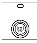
The rear window defogger uses a warming grid to remove fog from the rear window. Press the button to turn on the defogger. An indicator light will come on to remind you that the defogger is on. The defogger will turn off automatically after about 10 minutes of use. If you turn it on again, the defogger will operate for about five minutes only. You can also turn the defogger off by pressing the button again. The indicator light will go off when the system is turned off.
