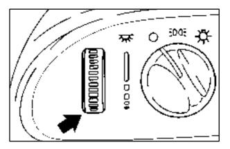
The thumbwheel controls the brightness of your instrument panel lights. Move the thumbwheel to brighten or dim the lights. If you move the thumbwheel all the way up, your courtesy lamps will come on.
