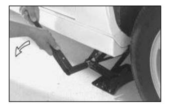
8. Lower the vehicle by turning the wheel wrench counterclockwise. Lower the jack completely.
