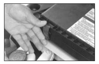
1. Unlatch the two clamps located on the front of the filter.
