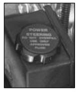
The power steering fluid reservoir is toward the rear of the engine, on the driver's side.
