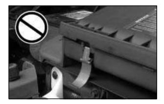
4. Close the cover without overlap (clamp will not latch with overlap) and latch the clamps.
