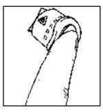
Press the button in to make your front and rear turn signal lamps flash on and off.
