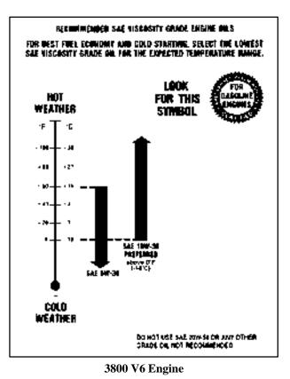
As shown in the chart, if you have the 3800 V6 engine, SAE 10W-30 is best for your vehicle. However, you can use SAE 5W-30 if it's going to be colder than  $60^{\circ}$ F (16°C) before your next oil change. When it's very cold, you should use SAE 5W-30. These numbers on an oil container show its viscosity, or thickness. Do not use other viscosity oils, such as SAE 20W-50.
