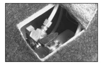
Open the hatch and find the tab along the driver's side trim panel. Lift up the tab and turn the valve counterclockwise to release the hydraulic pressure. Turn the ignition key to LOCK. You can now raise or lower your top manually. Be sure to close the valve after installing your top so you can raise or lower it electrically later.
