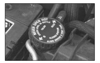
9. Then replace the pressure cap. At any time during this procedure if coolant begins to flow out of the filler neck, reinstall the pressure cap. Be sure the arrows on the pressure cap line up like this.
