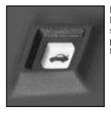
Press the button under the lamp control on the driver's side below the instrument panel to unlock the hatch from inside your vehicle.
