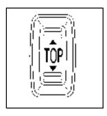
Make sure there is nothing or anyone on or around the top. Push and hold down the down arrow (▼) on the convertible TOP switch.
