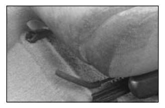
There are two levers at the front of the seat. The left lever adjusts the seat forward and rearward. The right lever adjusts the angle of the front of the seat.
