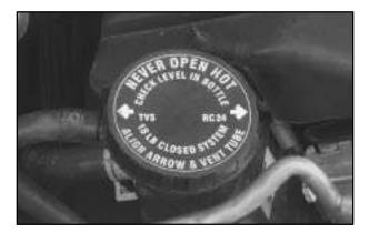
7. Shut the engine off and replace the pressure cap. Be sure the arrows on the cap line up like this.
