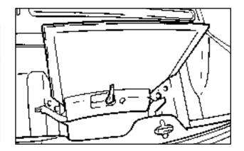
1. Open the cargo cover completely. Place the panel in the correct slot (DRIVER or PASSENGER) in the rear area of your vehicle. Make sure the handle is open and facing you when you put it in the storage slot.
