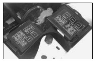
Look at the silver-colored band inside the fuse. If the band is broken or melted, replace the fuse. Be sure you replace a bad fuse with a new one of the correct size.
