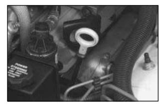
The engine oil dipstick is the yellow loop near the back of the engine.
