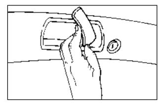
2. Then pull on the release handle to unlatch the panel. Lift the outer edge of the panel and pull it toward you. Then carry the panel to the rear of the vehicle for storage.
