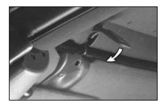
3. Pull down on the latches and align the hooks with the holes. Push forward on the larger part of the latch until it clicks. Do not force the latch. If it is hard to lock, the top is not properly aligned.
