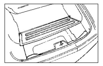
The cargo cover can be closed for hidden storage in the rear area of your vehicle. It can also help reduce noise in the vehicle when placed in the upright position, closing out the rear-end area.
