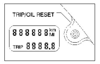
The trip odometer can tell you how far your car has been driven since you last set the trip odometer to zero.
