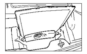
2. Push the handle closed to secure the panel in the slot. To lock each panel in the storage area, use your door key.
