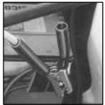
8. Now connect the black negative (-) cable to the good battery's negative (-) terminal.
