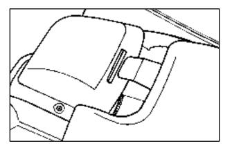
2. Remove the two side pieces of the boot cover by lifting the rear cover and sliding them out of their slots.
