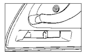
To lock the door from the inside, slide the lock control on the door rearward.
