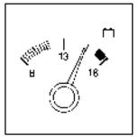
You can read battery voltage on your voltmeter. If it reads less than 11 volts or more than 16 volts while your engine is running, and it stays there, you may have a problem with the electrical charging system.
