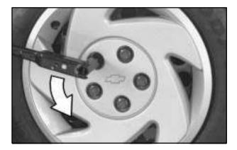
If your vehicle has a bolt-on wheel cover, loosen the plastic caps using the wheel wrench and remove the wheel cover.
