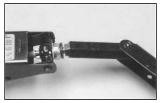
The jack has a bolt at the end. Attach the wheel wrench to the jack bolt.
