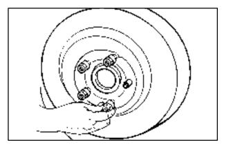
7. Replace the wheel nuts with the rounded end of the nuts toward the wheel. Tighten each nut by hand until the wheel is held against the hub.
