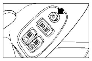
The power mirror control is on the driver's door. To adjust either mirror, turn the selector switch to L (left) or R (right). Then use the control to adjust the mirror.
