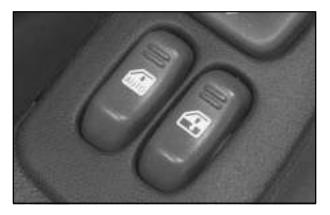
Switches on the driver's door control each window when the ignition is on or when RAP is present. (See "Retained Accessory Power" in the Index.) You can open the passenger's window any amount by pressing the switch and releasing it when the window has lowered to the position you want.
