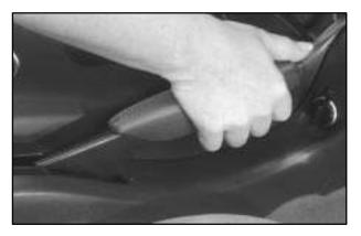
To release the parking brake, hold the brake pedal down. Pull the parking brake lever up until you can push in the release button. Hold the release button in as you move the brake lever all the way down.
