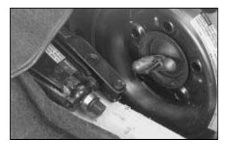
To remove the jack and wheel wrench, loosen and remove the plastic cover.
