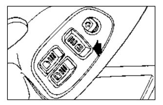
Press the power door lock switch located on the driver's door to lock or unlock both doors at once. Operating the power locks may affect the Content
