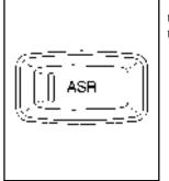
To turn the system off, press the ASR button located on the instrument panel.
