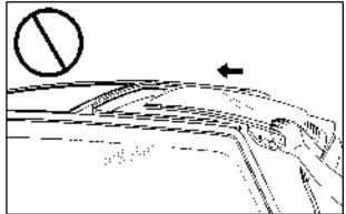
2. After the inboard edge of the panel is in position under the center roof rail, lower the outboard edge of the panel into position, close the latch and lock the T-top.
