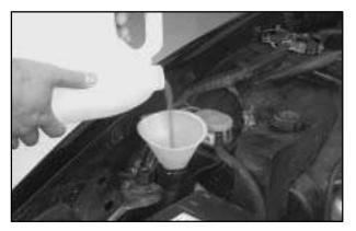
8. Then fill the coolant recovery tank to the proper level.
