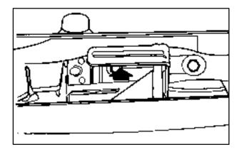
Then go to the front of the vehicle and pull up on the hood release located at the center area of the hood.
