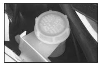
Refer to the Maintenance Schedule to determine how often you should check the fluid level in your clutch master cylinder reservoir and for the proper fluid. See "Owner Checks and Services" and "Recommended Fluids and Lubricants" in the Index.
