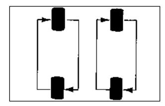
If you have P245/50ZR16 Goodyear Eagle GS-C tires or P275/40ZR17 Goodyear Eagle F1-GS tires, they must roll in a certain direction for the best overall performance. The direction is shown by an arrow on the sidewall. Because these tires are directional, they should be rotated as shown here. These tires should only be moved from front to rear and rear to front on the same side of the vehicle. Don't include the compact spare tire in your tire rotation.
