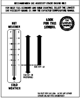
As shown in the chart, if you have the 5.7L V8 engine, SAE 5W-30 is best for your vehicle. However, you can use SAE 10W-30 if it's going to be  $0^{\circ}F$  (-18°C) or above. These numbers on an oil container show its viscosity, or thickness. Do not use other viscosity oils, such as SAE 20W-50.
