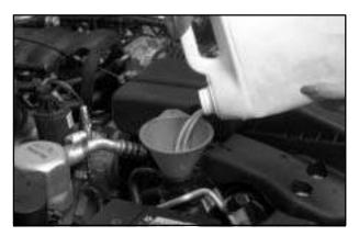
Fill the radiator with the proper DEX-COOL<sup>®</sup> coolant mixture, up to the base of the filler neck. (See "Engine Coolant" in the Index for more information about the proper coolant mixture.)
