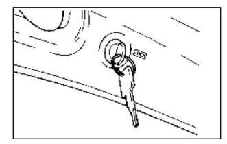
1. The door key unlocks the panels. The lock is over the door window. Turn the key counterclockwise to unlock the panel.
