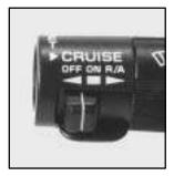
With cruise control, you can maintain a speed of about 25 mph (40 km/h) or more without keeping your foot on the accelerator.
