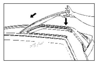
1. When installing the panels to the roof, keep the outboard edge of the panel raised about three inches (8 cm) above the roof while placing the inboard edge of the panel under the center roof.
