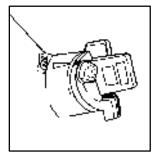
If you have a manual transmission, your ignition lock has a key release button. You must press the key release button to turn the ignition key to LOCK before you can take your key out.
