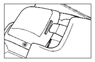
2. Remove the two side pieces of the boot cover by lifting the rear cover and sliding them out of their slots.
