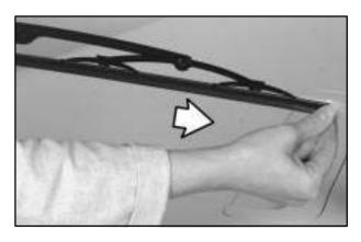
Hold the wiper blade assembly with one hand and pull the element gently with the other hand. (Replacement blade elements have three plastic caps which retain two metal flexor strips. Do not remove these caps before the element is installed.)
