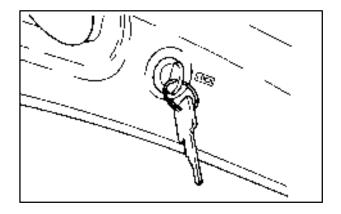
1. The door key unlocks the t-top panels. The lock is located over each door window. Turn the key counterclockwise to unlock the panel.
