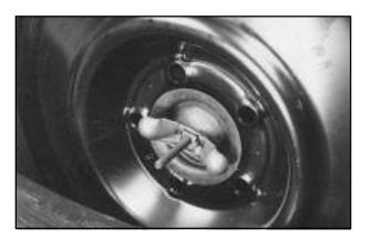
Remove the wing nut and adapter and pull out the spare.
