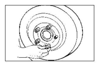
6. Install the spare tire and replace the wheel nuts with the rounded end of the nuts toward the wheel. Tighten each nut by hand until the wheel is held against the hub.
