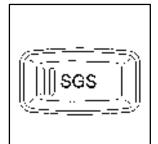
Your vehicle may be equipped with a Second-Gear Start feature. Press the Second-Gear Start (SGS) button located on the instrument panel to provide more traction when you are starting on ice or other slippery surfaces.
