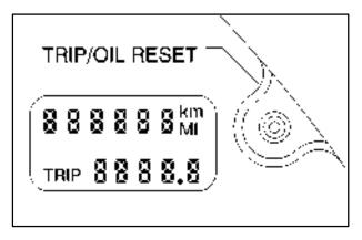
The trip odometer can tell you how far your car has been driven since you last set the trip odometer to zero.
