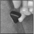
The front seatbacks fold forward to let people get into the back seat. To fold a seatback forward, lift the latch located on the lower backside of the seatback.
