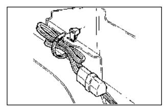
In very cold weather,  $0^{\circ}F$  (-18°C) or colder, the engine coolant heater can help. You'll get easier starting and better fuel economy during engine warm-up. Usually, the coolant heater should be plugged in a minimum of four hours prior to starting your vehicle.
