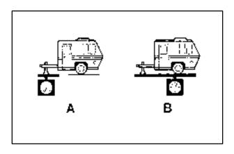
If you're using a weight-carrying hitch, the trailer tongue (A) should weigh 10 percent of the total loaded trailer weight (B). If you have a weight-distributing hitch, the trailer tongue (A) should weigh 12 percent of the total loaded trailer weight (B).
