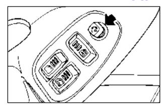
The power mirror control is located on the driver's door. To adjust either mirror, turn the selector switch to L (left) or R (right). Then use the control to adjust the mirror.
