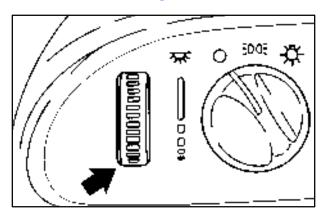
The thumbwheel controls the brightness of your instrument panel lights. Move the thumbwheel to brighten or dim the lights. If you move the thumbwheel all the way up, your courtesy lamps will come on.
