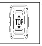
4. Push and hold the up arrow on top part of the convertible TOP switch.
