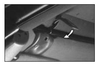
5. Pull down on the latches and align the hooks with the holes. Push forward on the larger part of the latch until it clicks. Do not force the latch. If it is hard to lock, the top is not properly aligned.
