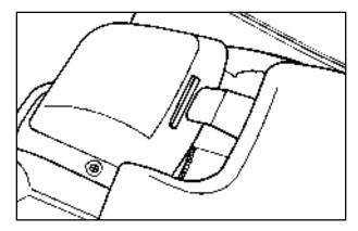
3. Install the two side covers by inserting the tab into the front seatbelt cover. Lower the covers onto the vehicle.
