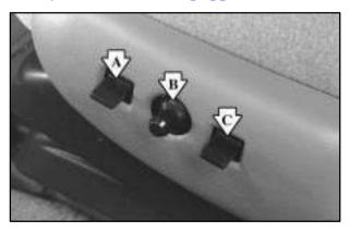
The driver's seat has three power seat controls located on the left side.
