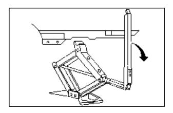
Position the jack under the vehicle. There is a notch in the vehicle's rocker flange on the coupe model. Raise the jack head until it fits firmly into the notch nearest the flat tire.
