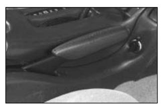
To set the parking brake, hold the brake pedal down and pull up on the parking brake lever. If the ignition is on, the brake system warning light will come on.
