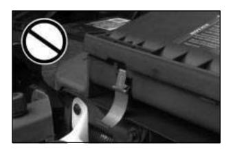
4. Close the cover without an overlap (clamp will not latch with an overlap) and latch the clamps.
