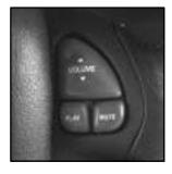
If your vehicle has this feature, you can control certain radio and compact disc functions using the buttons on your steering wheel.
