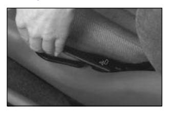
To adjust the seatback, lift the lever located on the outer side of the seat. Release the lever to lock the seatback where you want it. Pull up on the lever and the seat will go to its original upright position.
