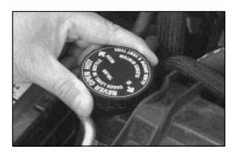
1. You can remove the radiator pressure cap when the cooling system, including the radiator pressure cap and upper radiator hose, is no longer hot. Turn the pressure cap slowly counterclockwise until it first stops. (Don't press down while turning the pressure cap.)
