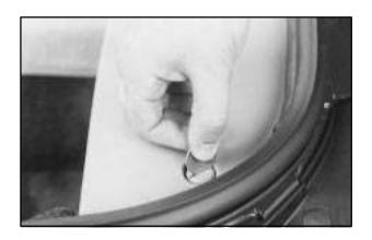
Find the plastic screw heads in the trim panel over the spare tire. See "Compact Spare Tire" later in this section for more information about the compact spare. Use a coin or a key to turn the screw heads until the slots point front and back to the unlock position. Gently lift the trim panel front forward edge and remove the panel.
