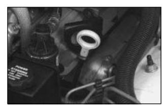
The engine oil dipstick is the yellow loop located near the back of the engine. Do not check the 5.7L V8 engine oil level after the engine has been sitting overnight. A higher than normal reading might be obtained. Check oil level with the oil warm.
