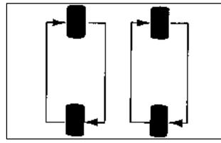
If you have P245/50ZR16 Goodyear Eagle GS-C tires or P275/40ZR17 Goodyear Eagle F1-GS tires, they must roll in a certain direction for the best overall performance. The direction is shown by an arrow on the sidewall. Because these tires are directional, they should be rotated as shown here. These tires should only be moved from front to rear and rear to front on the same side of the vehicle.
