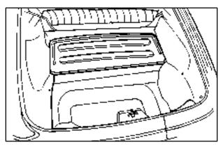
The cargo cover can be closed for hidden storage in the rear area of your vehicle. It can also help reduce noise in the vehicle when placed in the upright position, closing out the rear-end area.
