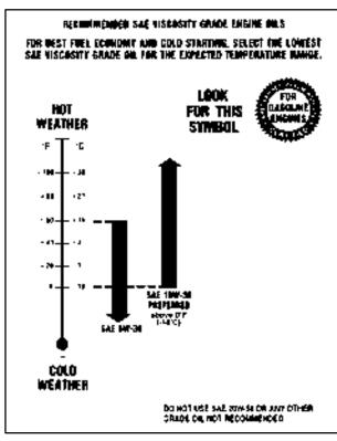
As shown in the chart, if you have the 3800 V6 engine, SAE 10W-30 is best for your vehicle. However, you can use SAE 5W-30 if it's going to be colder than 60°F (16°C) before your next oil change. When it's very cold, you should use SAE 5W-30. These numbers on an oil container show its viscosity, or thickness. Do not use other viscosity oils, such as SAE 20W-50.
