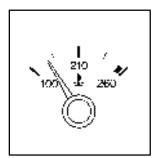
This gage shows the engine coolant temperature. If the gage pointer moves into the red area, your engine is approaching an overheating condition.
