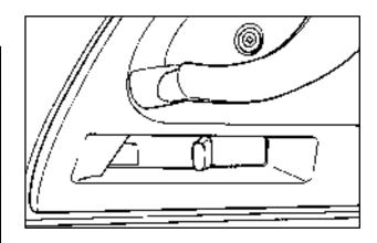
To lock the door from the inside, slide the lock control located on the door rearward.
