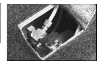
Open the hatch and find the tab located along the driver's side trim panel. Lift up the tab and turn the valve counterclockwise to release the hydraulic pressure. Turn the ignition key to LOCK. You can now raise or lower your top manually. Be sure to close the valve after installing your top so you can raise or lower it electrically later.
