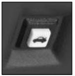
Press the button located under the lamp control on the driver's side below the instrument panel to unlock the hatch from inside your vehicle. If you have an automatic transmission, the shift lever must be in PARK (P) or NEUTRAL (N) to use the remote hatch release. If you have a manual transmission and the ignition is in RUN, you must set the parking brake before you can use the remote hatch release.
