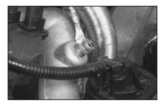
3. After the engine cools, open the coolant air bleed valve. There is one bleed valve. It is located on the thermostat housing.
