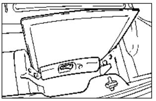
2. Push the handle down to close and secure the panel in the slot. To lock each panel in the storage area, use your door key.
