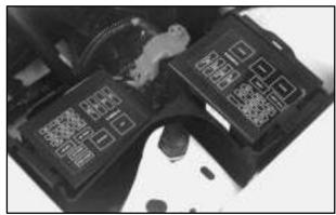
The other two are located in the engine compartment. Open the cover on either of the boxes to expose the fuses.
