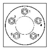
8. Tighten the wheel nuts firmly in a crisscross sequence as shown.
