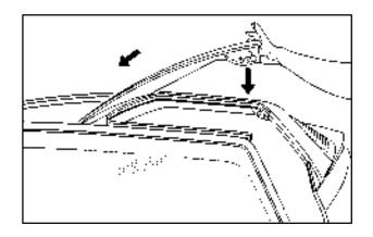
1. When installing the panels on the roof, keep the outboard edge of the panel raised about 3 inches (8 cm) above the roof while placing the inboard edge of the panel under the center of the roof.
