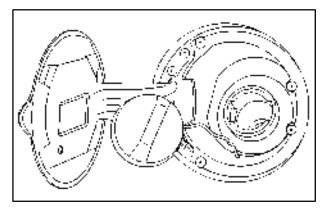
While refueling, hang the cap from the hook on the hinge. The lip of the cap will fit into the groove on the hook.
