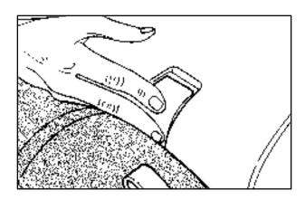
2. Remove the middle piece of the cover by pushing in on the latch and lifting up on the cover.
