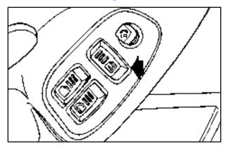
Press the power door lock switch located on the driver's door to lock or unlock both doors at once.
