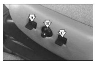
The driver's seat has three power seat controls located on the outboard side.
