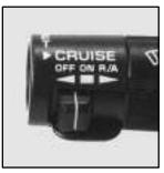
With cruise control, you can maintain a speed of about 25 mph (40 km/h) or more without keeping your foot on the accelerator.
