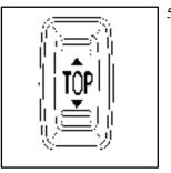
5. Make sure there is nothing or anyone on or around the top. Push and hold the down arrow on the lower part of the convertible TOP switch.
