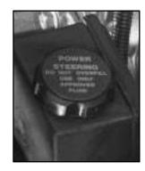
The power steering fluid reservoir is located toward the front of the engine, on the driver's side. See "Engine Compartment Overview" in the Index for more information on location.
