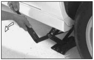
7. Lower the vehicle by turning the wheel wrench counterclockwise. Lower the jack completely.
