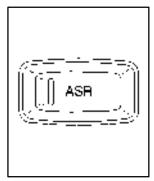
To turn the system off, press the ASR button located on the instrument panel.
