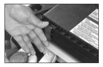
1. Unlatch the two clamps located on the front of the filter.
