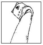
Press the button on the steering column in to make your front and rear turn signal lamps flash on and off.
