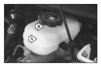
You can check the brake fluid without taking off the cap. Just look at the brake fluid reservoir. The fluid level should be above the plastic seam in the reservoir (A). If it isn't, have your brake system checked to see if there is a leak.
