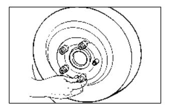
6. Install the compact spare tire and put the wheel nuts back on with the rounded end of the nuts toward the wheel. Tighten each nut by hand until the wheel is held against the hub.
