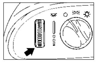
The thumbwheel controls the brightness of your instrument panel lights. Move the thumbwheel up or down to brighten or dim the lights. If you move the thumbwheel all the way up, your courtesy lamps will come on.
