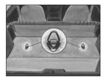
If you have a convertible, don't use a child restraint with a top strap in your vehicle because the top strap anchor cannot be installed properly. You shouldn't use this type of restraint without anchoring the top strap.
