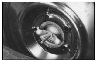
4. Remove the wing nut and adapter and pull out the compact spare tire.
