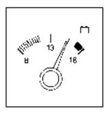
You can read the battery voltage on your voltmeter. If it reads less than 11 volts or more than 16 volts while your engine is running, and it stays there, you may have a problem with the electrical charging system.
