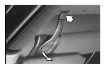
4. Unlock the front of the convertible top by pushing on the smaller part of the latch, then pulling down on the larger part of the latch. Be sure the hook on the latch that attaches into the hole at the windshield releases.
