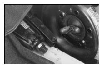
3. To remove the jack and wheel wrench, loosen and remove the plastic cover.
