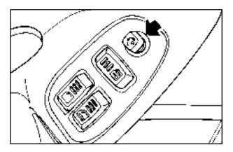
The power mirror control is located on the driver's door. To adjust either mirror, turn the selector switch to L (left) or R (right). Then push the control in the direction you want the mirror to go.
