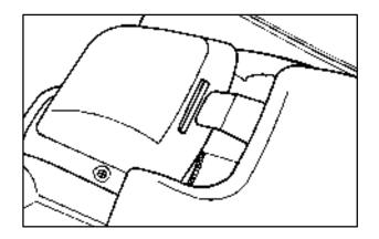
Install the two side covers by inserting the tab into the front seatbelt cover. Lower the covers onto the vehicle.
