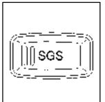
Your vehicle may be equipped with a Second-Gear Start feature. Press the Second-Gear Start (SGS) button located on the instrument panel to provide more traction when you are starting on ice or other slippery surfaces.
