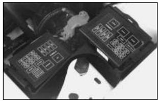
The other two are located in the engine compartment on the driver's side. Open the cover on either of the boxes to expose the fuses.
