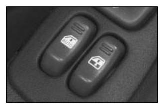
Switches on the driver's door control each window when the ignition is on or when Retained Accessory Power (RAP) is active. (See "Retained Accessory Power" in the Index.)
