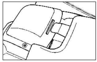
3. Remove the two side pieces of the boot cover by lifting the rear cover and sliding them out of their slots.
