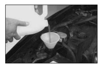
8. Then fill the coolant recovery tank to the proper level.
