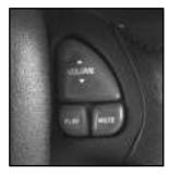
If your vehicle has this feature, you can control certain radio and compact disc functions using the buttons on your steering wheel.
