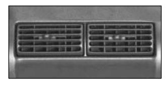
Adjust the direction of airflow by moving the vents.
