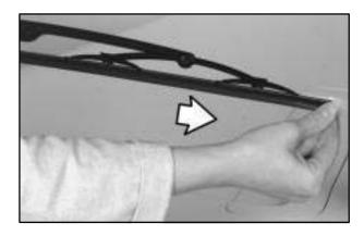
Hold the wiper blade assembly with one hand and pull the element gently with the other hand.
