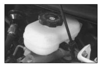
Your brake master cylinder reservoir is on the driver's side of the engine compartment. See "Engine Compartment Overview" in the Index. It is filled with DOT-3 brake fluid.
