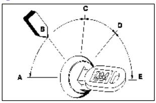
With the key in the ignition, you can turn the switch to five different positions.
