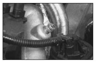
3. After the engine cools, open the coolant air bleed valve.
