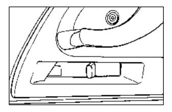
To lock the door from the inside, slide the lever located on the door rearward.
