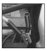
8. Now connect the black negative (-) cable to the good battery's negative (-) terminal.
