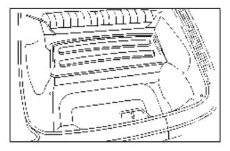
The cargo cover can be closed for hidden storage in the rear area of your vehicle. It can also help reduce noise in the vehicle when placed in the upright position, closing out the rear area.
