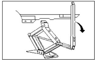
2. Position the jack under the vehicle. There is a notch in the vehicle's rocker flange on the coupe model. Raise the jack head until it fits firmly into the notch nearest the flat tire.
