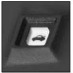
Press the button located under the main lamp control on the driver's side below the instrument panel to unlock the hatch from inside your vehicle. If you have an automatic transmission, the shift lever must be in PARK (P) or NEUTRAL (N) to use the remote hatch release. If you have a manual transmission and the ignition is in RUN, you must set the parking brake before you can use the remote hatch release.
