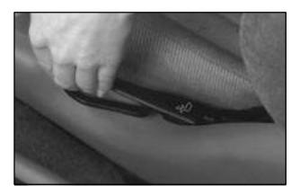
To adjust the seatback, lift the lever located on the outboard side of the seat. Release the lever to lock the seatback where you want it. Pull up on the lever and the seat will go to its original upright position.
