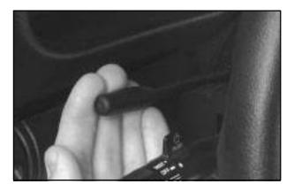
To tilt the wheel, hold the steering wheel and pull the lever toward you. Move the steering wheel to a comfortable level, then release the lever to lock the wheel in place.
