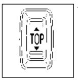
4. Push and hold the up arrow on the top part of the convertible TOP switch.
