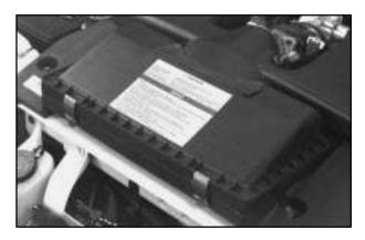
The engine air cleaner/filter is located at the front in the center of the engine compartment. See "Engine Compartment Overview" in the Index for more information on location
