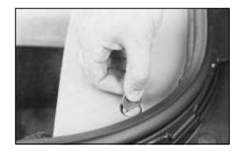
2. Find the plastic screw heads in the trim panel over the spare tire. See "Compact Spare Tire" later in this section for more information about the compact spare. Use a coin or a key to turn the screw heads until the slots point front and back to the unlock position. Gently lift the trim panel front forward edge and remove the panel.
